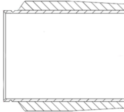
**Figure 3: Soleras tapered target design with chamfered target end design**
