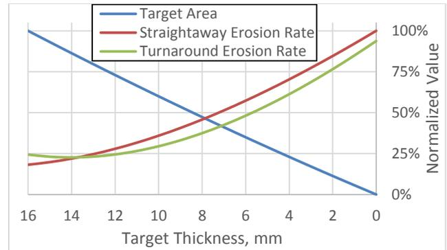
**Figure 2: Normalized target cross-sectional area and erosion rate as a function of the target thickness for a straight target run in metal mode**
