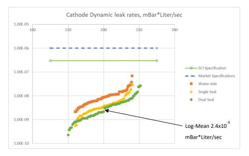
**<u>Conclusions</u>** – At SCI, we strive to continuously improve the capability and performance of our products and systems. By refining product leak testing procedures, we can demonstrate world class product performance and give customers and partners peace-of-mind for the integrity of the components they count on in their applications.
